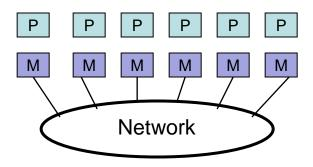
Distributed memory: each processor has its own local memory. Must do message passing to exchange data between processors. cc-NUMA enables larger number of processors and shared memory address space than SMPs; still easy to program, but harder and more expensive to build. (example: Clusters)
